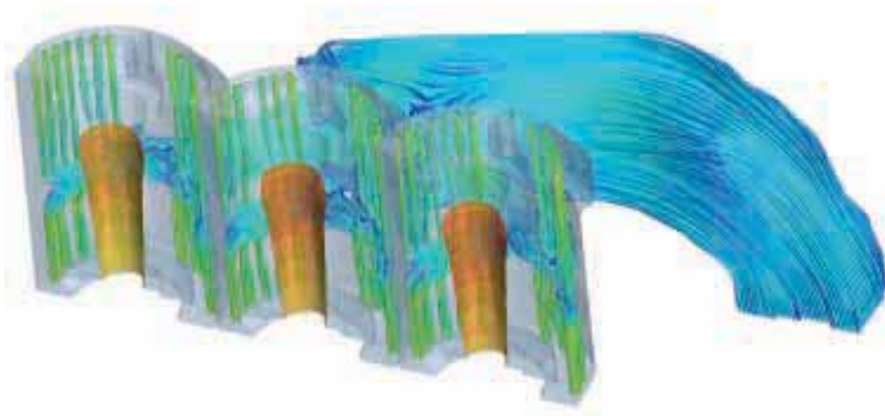
Conjugate heat transfer analysis: cooling
